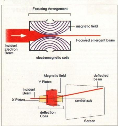
This diagram show the general layout of a cathode ray tube similar to that usually found inside an oscilloscope
